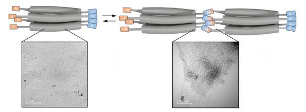
Figure 1. Top: schematic representation of the proposed assembly of coiled coil oligomers into nanostructures. Bottom: TEM images show reversible fiber assembly and disassembly via dynamic covalent chemistry.
